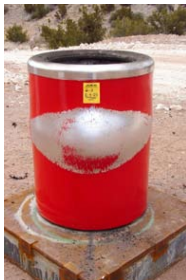
▲ BBC LITTER BIN the bin remains intact, instead of becoming a vehicle for the bomb
